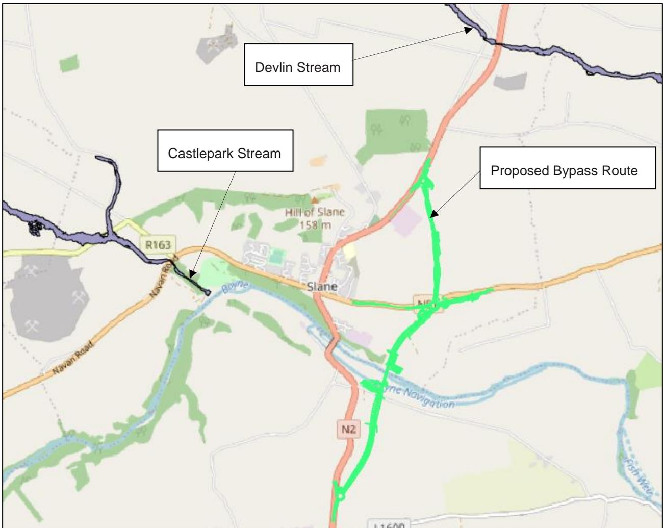
**Figure 3-11 NIFM Predictive Flood Mapping in vicinity of Proposed Bypass Route**
